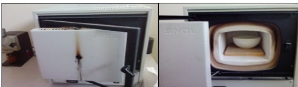
Fig. 4. Muffle Furnace used for determination of volatile matter, ash and fixed carbon content
