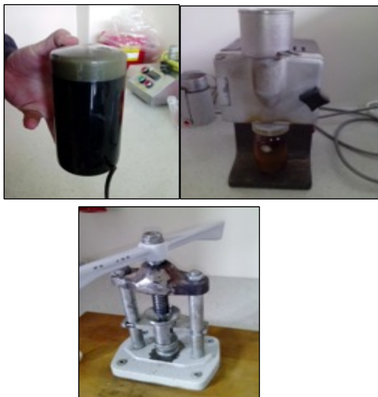
Fig. 6. Mini Shredder (right), Laboratory Mill (left) and Manual Presser used for shredding and pressing the of samples
