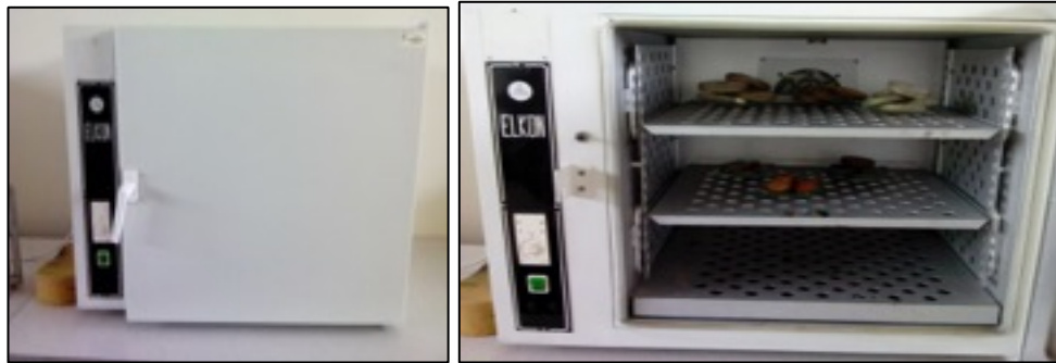
Fig.3. Lab Furnace used for determination of moisture content in the materials
