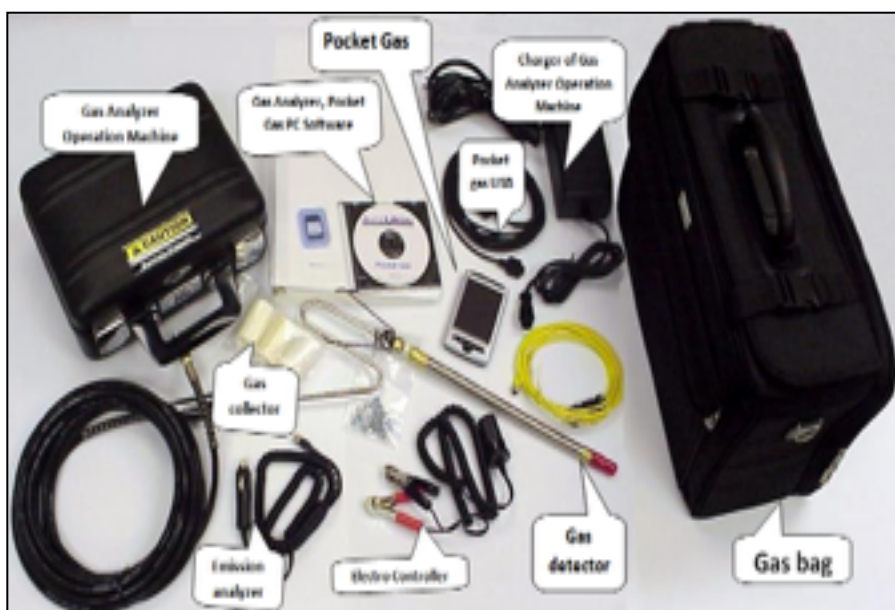
Fig. 13. Appearance and Naming of Gas Analyzer Pocket Gas.
